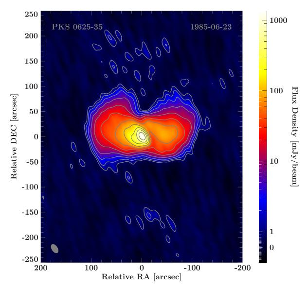
Figure 3.20.: VLA image of 0625-354 observed at 1.5 GHz in C-configuration. RMS: 0.33 mJy, map-peak: 1.36 Jy, beam:  $(19.5 \times 11.5)$  arcsec at 39.2°. Smallest contourlevel at three times RMS for positive and negative fluxdensities. The other contours changing exponential with base 2 in the positive fluxdensity regime. A bright core is visible and a FR1 like extended emission with an overall size of  $s \approx 200$  arcsec.
