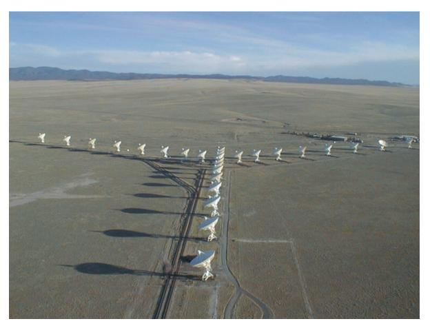
Figure 1.9.: Image of the whole VLA at D-configuration with maximal baselines of 1.03 km. Credits: Image courtesy of NRAO/AUI
