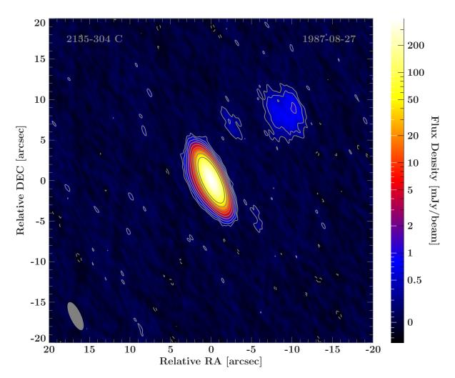
Figure 3.29.: Tapered VLA image of 2155-304 observed at 4.8 GHz in A-configuration. RMS: 0.084 mJy, map-peak: 0.389 Jy, beam:  $(3.71 \times 1.28)$  arcsec at 25.2°. Smallest contourlevel at three times RMS for positive and negative fluxdensities. The other contours changing exponential with base 2 in the positive fluxdensity regime. bright core is visible and an emission region in north western direction. up to about  $d_{\rm core} \approx$ 15 arcsec.
