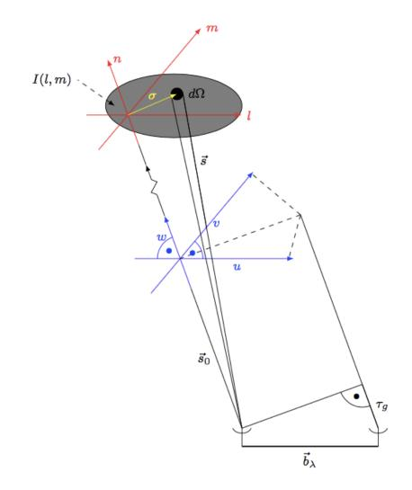
Figure 1.8.: Sketch of the different coordinate-systems used to explain radio interferometry of two antennas with sapcing of one baseline  $b_{\lambda}$ . The radiation arrives at the right antenna with a geometrical delay of  $\tau_g$  according to the left reference antenna. The grey emission area from which the radiation of he object comes from is given in coordinates l,m,n and the baselines of the array is represented by the u,v,w coordinated. Figure by Burd (2017).
