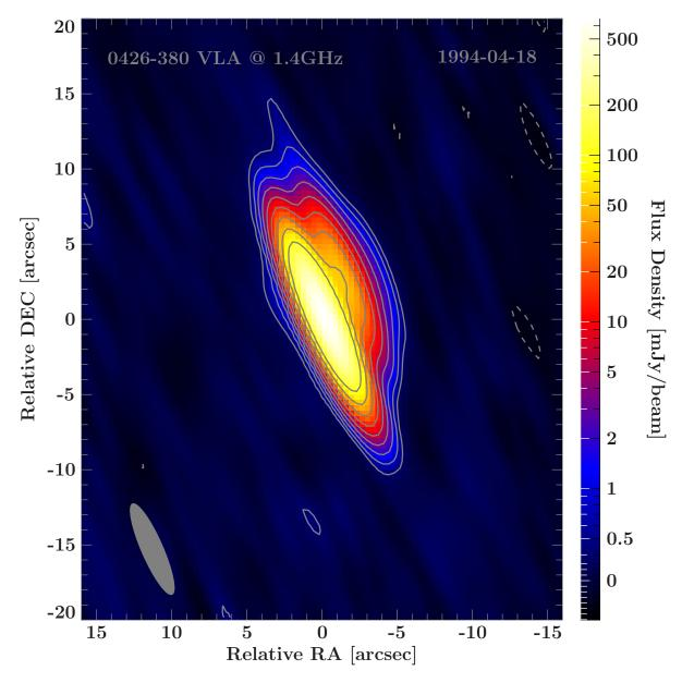
Figure 3.8.: VLA image of 0426-380 observed at 1.5 GHz in A-configuration. RMS: 0.14 mJy, map-peak: 0.663 Jy, beam:  $(6.57 \times 1.41)$  arcsec at 23.6°. Smallest contourlevel at three times RMS for positive and negative fluxdensities. The other contours changing exponential with base 2 in the positive fluxdensity regime. A bright core is visible and a jet extending up to  $d_{\text{core}} \approx 5 \operatorname{arcsec}$  in north western direction.
