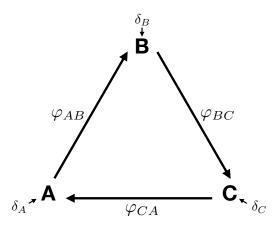
Figure 2.1.: Illustration for the explanation of the closure phases. A, B, C represent three telescopes of the considered array, the arrows the signal flux between the antennas.  $\varphi_{AB}$ ,  $\varphi_{BC}$  and  $\varphi_{CA}$  are the phases of two considered telescopes.  $\delta_A$ ,  $\delta_B$  and  $\delta_C$  represent the errors introduced by every single telescope.
