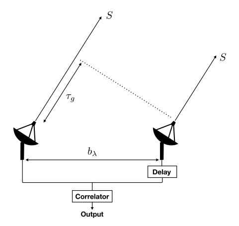
Figure 1.7.: Scheme of a two element interferometer, with two single-dish telescopes pointing in the direction of S with baseline  $b_{\lambda}$  and geometrical time-delay  $\tau_g$  between the to telescopes. Also an instrumental delay and the correlator is shown.
