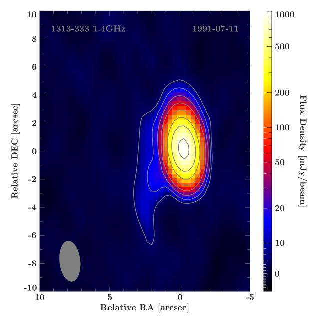
Figure 3.26.: VLA image of 1313-333 observed at 1.4 GHz in A-configuration. RMS: 2.2 mJy, map-peak: 1.02 Jy, beam:  $(2.89 \times 1.46)$  arcsec at 5.85°. Smallest contourlevel at three times RMS for positive and negative fluxdensities. The other contours changing exponential with base 2 in the positive fluxdensity regime. A bright core is visible and an extension in eastern direction.
