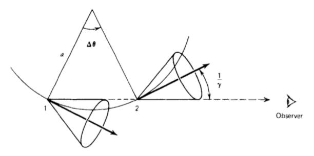
Figure 1.4.: Illustration of the beamed synchrotron radiation of a single electron with a relativistic circulation arround a magnetic field. The radiation is emitted in a cone with opening angle  $\theta$ . Credits: Rybicki & Lightman (1979).
