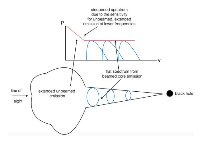
Figure 1.6.: Illustration of the composition of a blazar spectrum, consisting of a flat spectrum part caused by the beamed core emission and the steep part of the spectrum caused by the unbeamed extended emission of the source. The flat part of the spectrum is the result of the superpossition of the beamed spectra of single emission regions of the jet, peaking at different frequencies. Adapted from Burd (2017).
