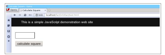
Figure 2.7: Screenshot of a demonstration website. A simple JavaScript example on a website that can calculate the square of a number inserted in the input field.
