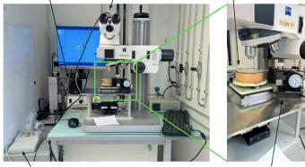
XYZ piezoelectric high precision positioning stage
