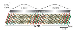
FIG. 1 (color online). (bottom panel) Schematic spin structure of the Mn monolayer on W(110). Nearest neighbor spins are slightly canted resulting in a cycloidal spin spiral with alternating out-of-plane and in-plane regions which repeat with a period of about 6 nm. (top) Spin-orbit coupling leads to an enhanced (reduced) LDOS over in-plane (out-of-plane) magnetized regions which can be detected with nonmagnetic tips.
