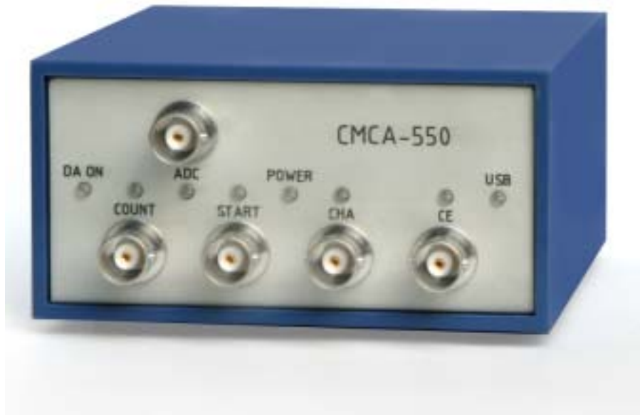
Fig.1a Front view of the CMCA-550 Data Acquisition Module The front panel is equipped with five BNC connectors for the analog input ADC and the digital inputs COUNT, START, CHA and CE and with eight LED's showing the actual status of the Data Acquisition Module
