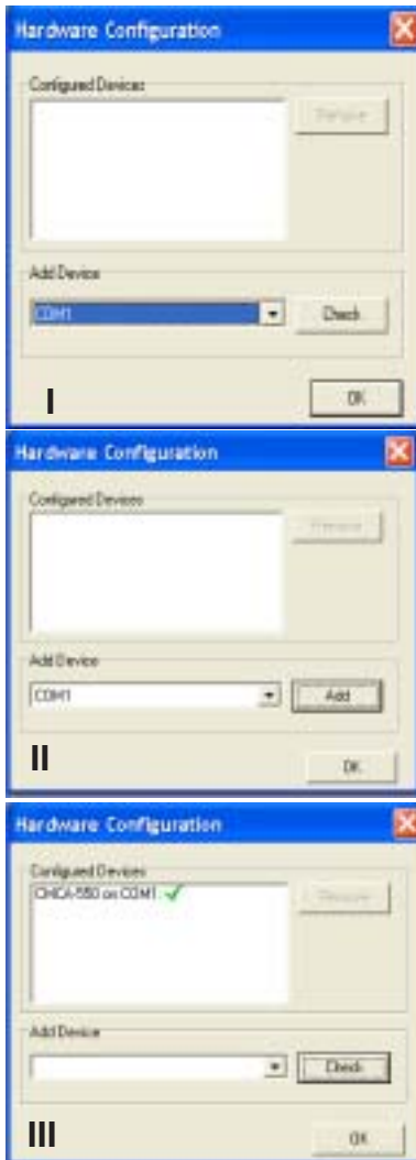
Fig. 11b Wissoft 2003 the Hardware Configuration Panel for Adding a Data Acquisition Unit
