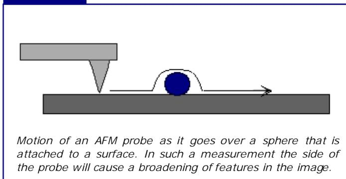
Often the size of features on the surface such as nanotubes or nanospheres look larger than expected. However, the height of the feature when measured by a line profile is correct.
