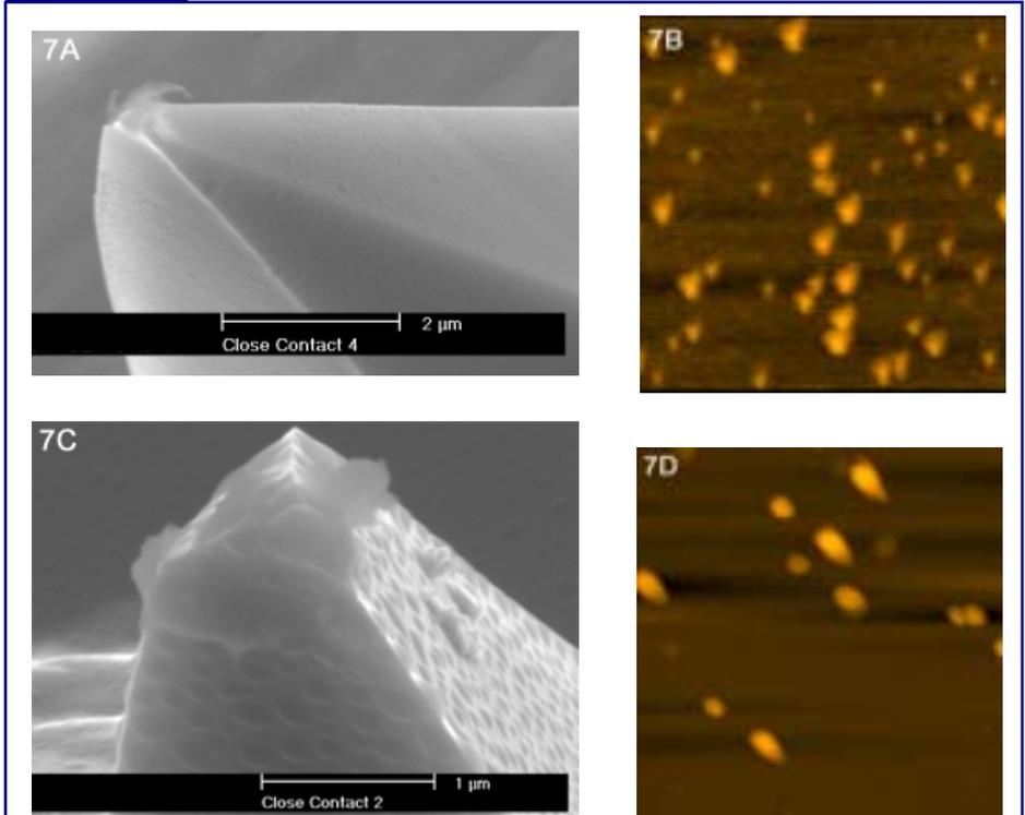
The AFM images at the right, B (5 nm in diameter) and D (28 nm in diameter), are of nanospheres that are supposed to be perfect spheres. At the right, A and C, are scanning electron microscope images of the AFM probes used for getting the images of the spheres. Because the chipped probes are much larger than the spheres, the AFM images reflect the probe's geometry. The scan size is 700nm X 700nm.
