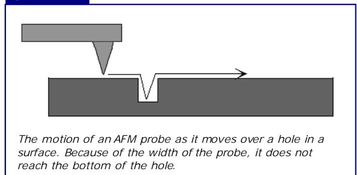
If the probe needs to go into a feature that is below the surface, the size of the feature can appear too small. The line profile in these cases is established by the geometry of the probe and not the geometry of the sample. However, it is still possible to measure the opening of the hole from this type of image. Also, the pitch of repeating patterns can be accurately measured with probes that don't reach the bottom of the features being imaged.
