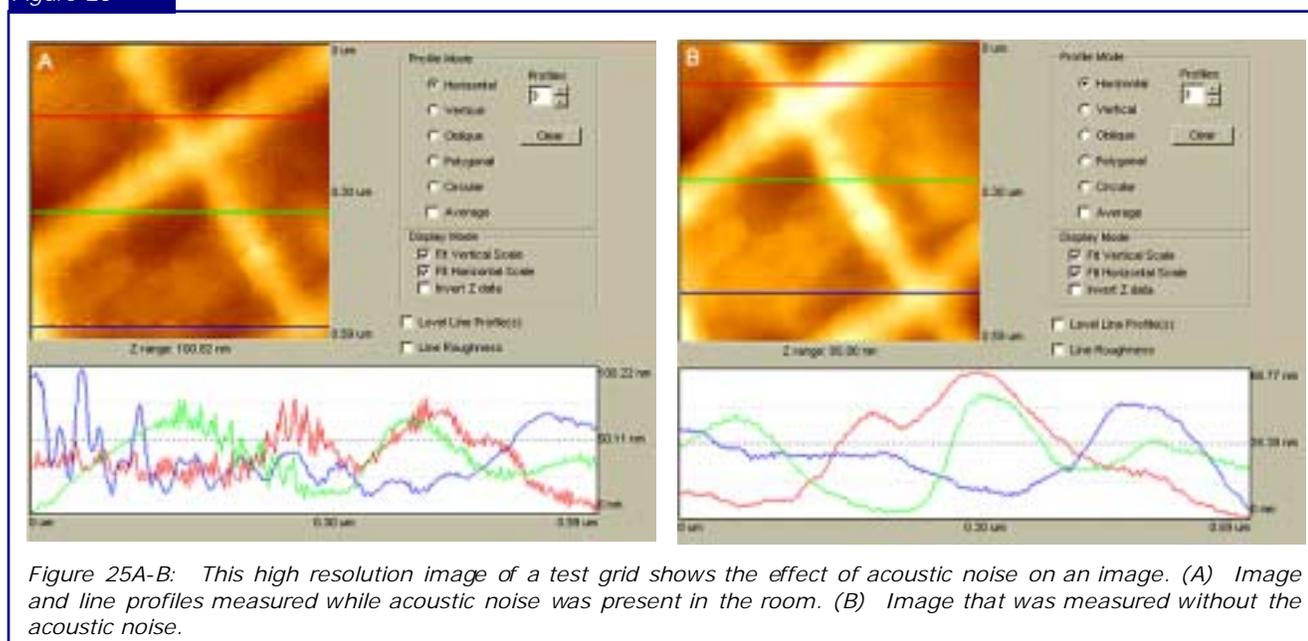
Figure 25A-B: This high resolution image of a test grid shows the effect of acoustic noise on an image. (A) Image and line profiles measured while acoustic noise was present in the room. (B) Image that was measured without the acoustic noise.
