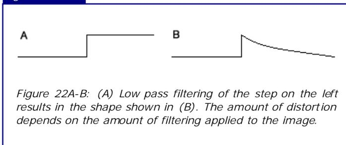
When images are viewed that have substantial low pass filtering, the dimensions in the image can appear distorted. Other artifacts can appear as a sharpness at the edge of steps in an image.
