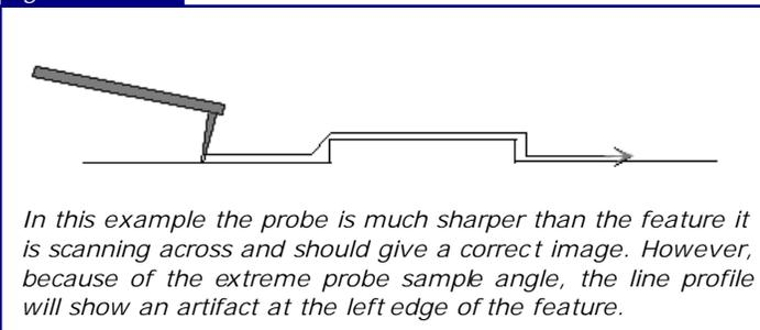
Solving this problem is achieved by adjusting the angle between the probe and the sample so that they are perpendicular. In some microscopes the probe is designed to be at a 12 degree angle with respect to the sample. Also some AFM microscopes do not have mechanical adjustments to control the probe/sample angle.
