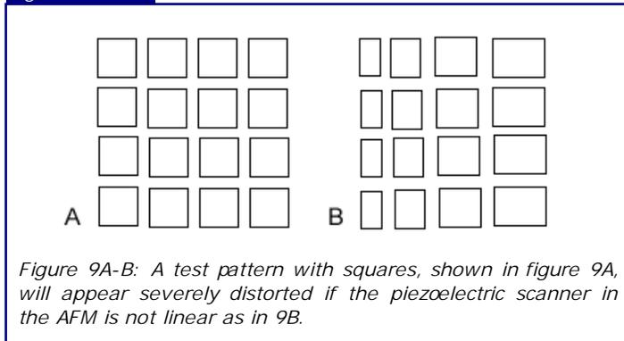
Once the scanner is properly linearized, it is also critical that the scanner be calibrated. For example it is possible for the scanner to be linear but not calibrated. If the calibration is incorrect, then the X-Y values measured from line profiles will be incorrect.
