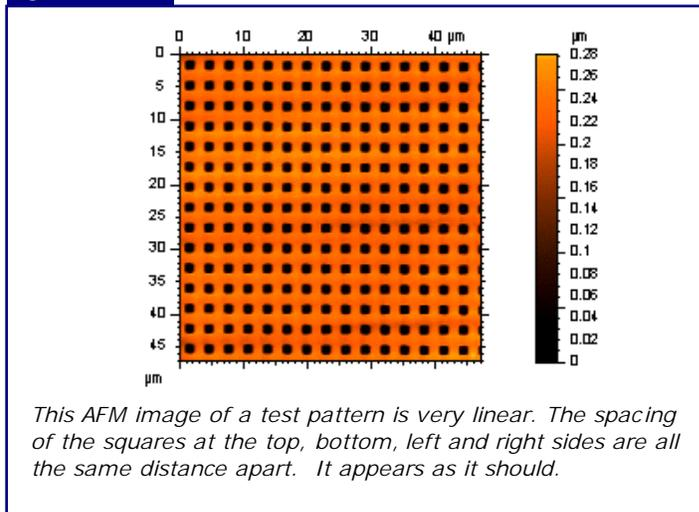
A common method for correcting the problems of X-Y non-linearity and calibration is to add calibration sensors to the X-Y piezoelectric scanners. These sensors can be used to correct the linearity and the calibration in real time.
