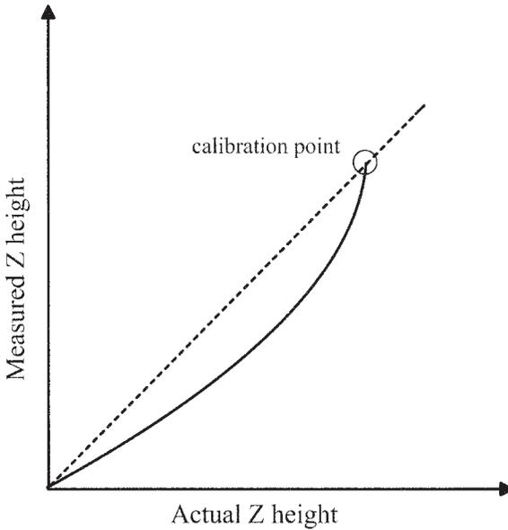
Fig. 7. Quite often, the  $z$  height response of the scanner is calibrated in only one point. The plot represents the deviation from the true value for measurement of heights that differ from the one at which the scanner has been calibrated.
