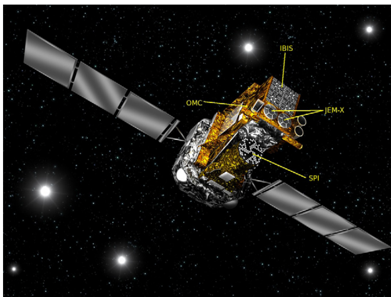
Figure 2.1: Artist impression of INTEGRAL with its instruments labeled; picture from (Diehl, 2013)
