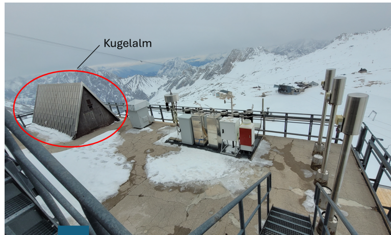
Fig. 4.2: The Kugelalm houses several scientific instruments. The detector used in the simulations is located inside the Kugelalm, shielding it from the weather.
