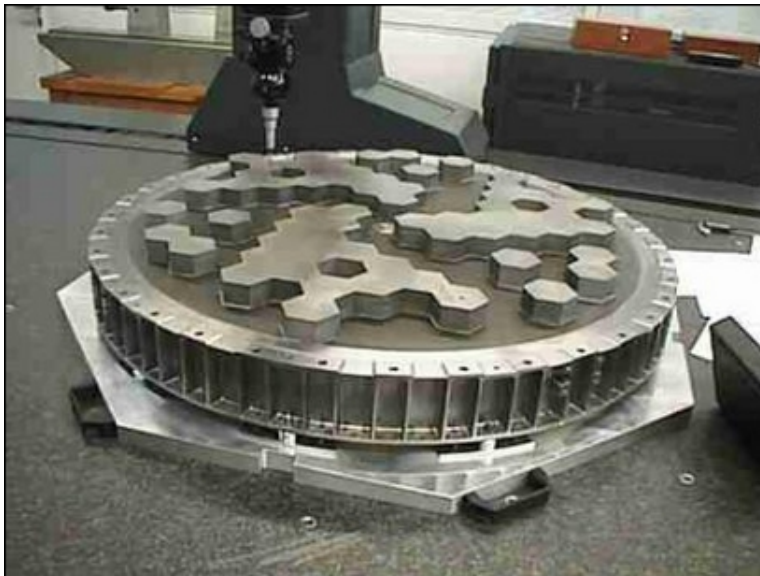
Figure 3.5: The tungsten mask shielding the Germanium detector camera. From Dubath et al. 2005.
