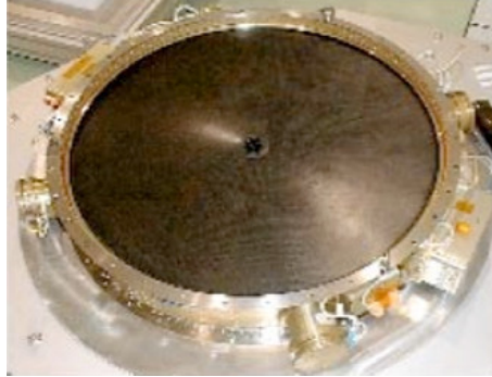
Figure 4.4: The plastic scintillator anticoincidence subassembly (PSAC) below the tungsten mask for reducing the background at 511 keV. From [32].
