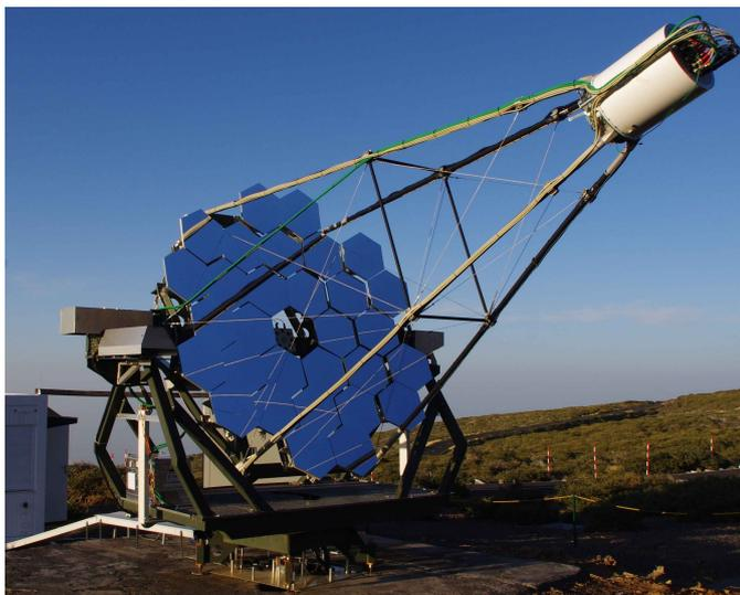
**Figure 4.5:** The FACT telescope at 2,200 m altitude on La Palma. The  $9.5 \text{ m}^2$  mirror area focuses the Cherenkov light of air shower particles in the camera with G-APD photo sensors. Image from Anderhub et al. (2013a).
