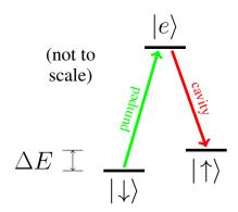
• Applied magnetic field shifts the hyperfine states unequally, so a linear gradient in *B* provides a site-dependent shift in energy, say in  $|\downarrow\rangle$  but not  $|\uparrow\rangle$ .
