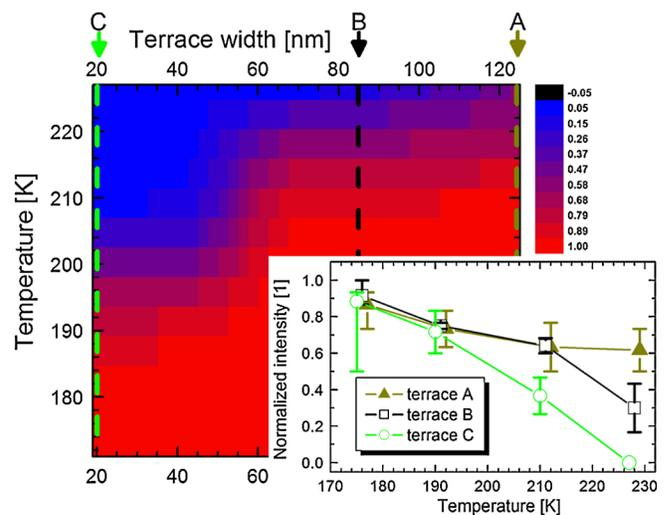
FIG. 4 (color online). Color-coded peak intensity at an inverse periodicity of  $0.16 \text{ nm}^{-1}$  as found on nine terraces in Fig. 3. The inset shows the peak intensity found on terraces A, B, and C after normalization at 40 K.
