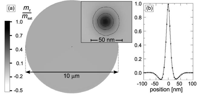
FIG. 1. (a) Calculated gray-scale plot and (b) line profile of  $m_z$  in the central region of a 30 nm thick polycrystalline Co disk ( $d = 10 \mu\text{m}$ ). Inset: magnified region around the vortex core which appears as a tiny black dot in (a) [10].
