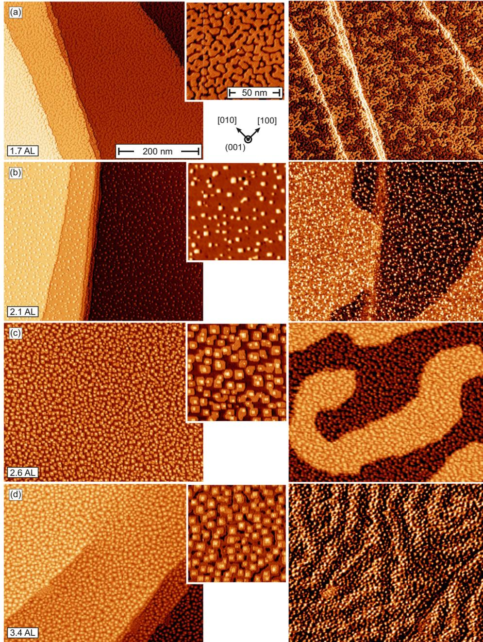
FIG. 4. (Color online) Coverage-dependent topographic STM images showing an overview (left panel) and a zoomed-in (middle) along with the magnetic domain structure as obtained by SP-STM (right) of Fe films on Rh(001): (a) 1.7 AL (scan parameters:  $U = -0.6$  V,  $I = 1.5$  nA), (b) 2.1 AL ( $U = -0.7$  V,  $I = 3.0$  nA), (c) 2.6 AL ( $U = -0.7$  V,  $I = 1.5$  nA), and (d) 3.4 AL ( $U = -0.5$  V,  $I = 2.5$  nA).
