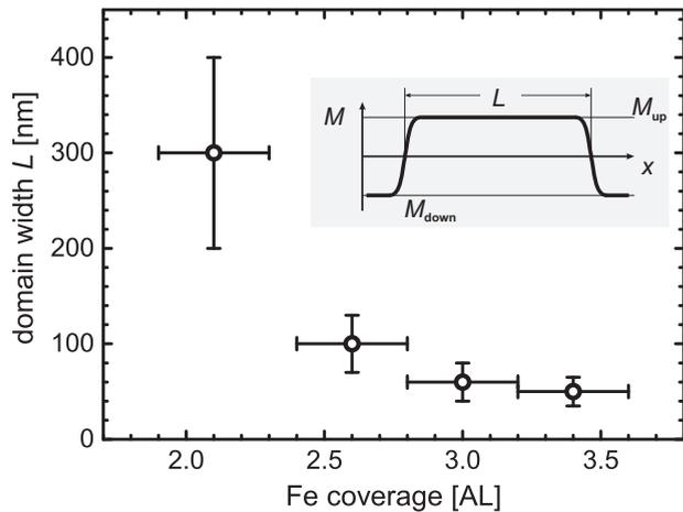
FIG. 5. Coverage dependence of the stripe domain width  $L$  versus coverage observed for Fe/Rh(001).
