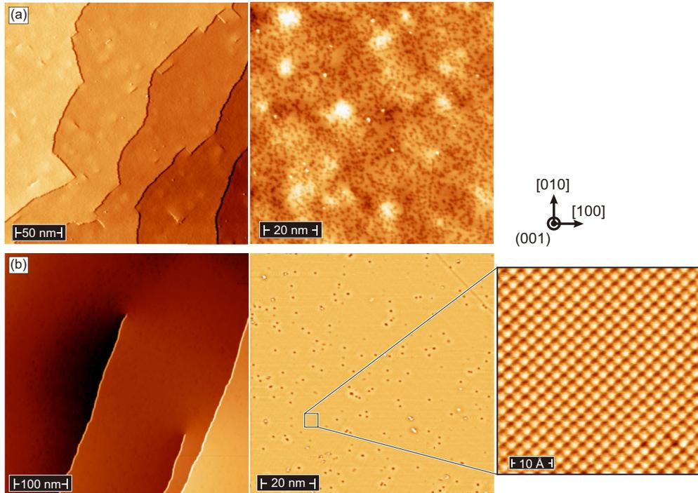
FIG. 1. (Color online) Topographic STM images of the bare Rh(001) surface as prepared by different procedures: (a) by sputtering and annealing and (b) with additional oxygen treatment (see text for details). While the surface contains numerous defects in (a), which probably originate from carbon, a very low defect density is observed in (b). Scan parameters:  $U = +1$  V,  $I = 200$  pA (atomic resolution:  $U = +2$  mV,  $I = 10$  nA).
