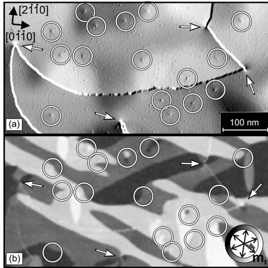
FIG. 1. (a) STM topograph and (b) magnetic signal map of a 90 AL Dy film. The schematic inset summarizes the different magnetic contrast levels which result from different projections of  $m_s$  onto  $m_t$  calculated as in Ref. 4. The arrows (circles) mark the position where screw (edge) dislocation appear on the surface.
