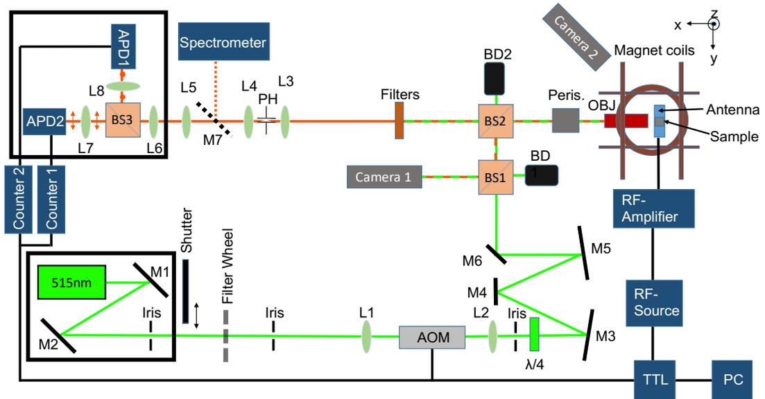
Figure 3.1.: The optical table. M: silver coated mirror; L: lens; BD: beam dump; BS beam splitter; OBJ: microscope objective; PH: pin hole ( $15 \mu\text{m}$  diameter); Peris: periscope.
