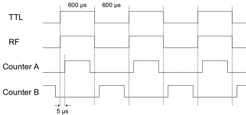
Figure 3.2.: The principle of gated photon counting.
