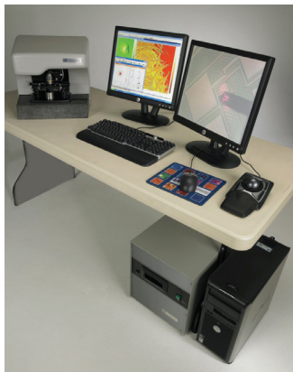
FIGURE 2-1 Photograph of a table top AFM illustrating the major components. They are a microscope stage, computer, electronic controller, computer monitor, and optical microscope monitor. The trackball is used for moving the sample stage in the X-Y axis. Most of the AFMs in use in laboratories around the world are table top units such as this. Resolution can often be enhanced by placing the microscope stage on a vibration isolation table.
