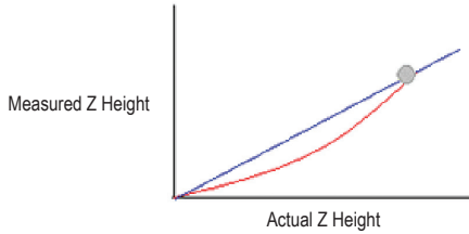
FIGURE 6-11 This graph shows the relationship between an actual Z height and a measured Z height in an atomic force microscope. Often only one calibration point is measured as shown by the grey circle, and the Z ceramic is assumed to be linear, as shown by the blue line. However, as is often the case, the ceramic is nonlinear, as shown by the red line. In such cases incorrect Z heights are measured with the microscope unless the feature being measured is close to the calibration measurement.
