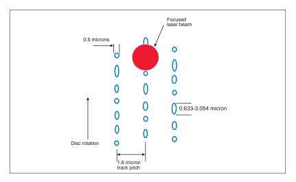
Figure 2: Compact disc data surface.
