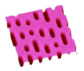
Figure 1: TappingMode<sup>TM</sup> AFM image of CD surface.  $10\mu m$  scan.
