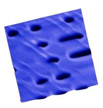
Figure 7: An example of pit smearing leading to poor playability on an audio CD. 7.3µm scan.
