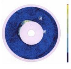
Figure 9: BLER map of the disc in Figure 8 (very high BLER indicated in yellow).
