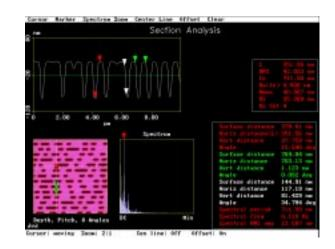
*Figure 5: Cross-sectional analysis of DVD disc (Figure 4b).*
