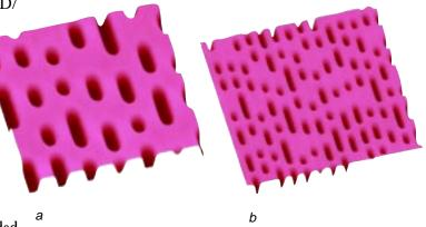
Figure 6: TappingMode AFM perspective images of a) CD disc and (b) DVD disc. 10μm scans.
